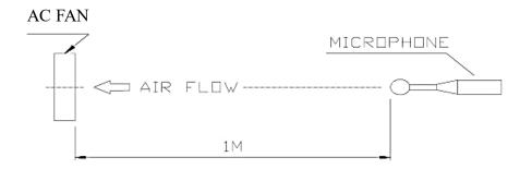
4. NOISE IS MEASURED AT RATED VOLTAGE IN FREE AIR IN A SEMI-ANECHOIC CHAMBER WITH A & D SOUND LEVEL METER WITH MICROPHONE AT A DISTANCE OF ONE METER FROM THE FAN INTAKE.
