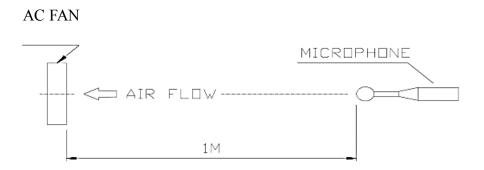
4. NOISE IS MEASURED AT RATED VOLTAGE IN FREE AIR IN A SEMI-ANECHOIC CHAMBER WITH A & D SOUND LEVEL METER WITH MICROPHONE AT A DISTANCE OF ONE METER FROM THE FAN INTAKE.
